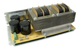
The PSA80V4A-1 power supply has a single 80V output, a voltage input of 115 or 220VAC, and power capabilities of up to 320 watts. With an unregulated output and a size of 8.30" x 4.25" x 2.81" and dual mounting position "L Bracket," the PSA80V4A-1 can be mounted just about anywhere. The PKG-343-MBC12-PS-CBL includes two wires for powering the MBC12101.
